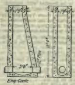
Fig. 27.—Concrete Manhole.
